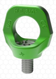
PLEASE NOTE: Hoist Eye 360® is suitable for applications where all lifting-eye rotation takes place before lifting begins, with no swivel action occurring while under load. For applications that require swiveling under load, use a Swivel Hoist Ring instead.
